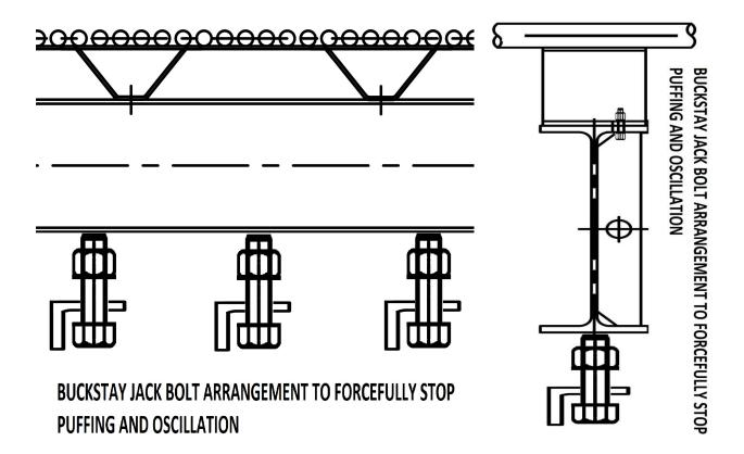
This type of correction does not follow the basic engineering guidelines for any type i.e. Hot Buckstay OR Cold Buckstay and the provided correction is like eyewash to avoid cost implication and get a new business again. As we know that, BUCKSTAY is designed for furnace pulsation & gas pressure fluctuation (Positive/Negative) and to control the movement & vibration of furnace water wall panels.
